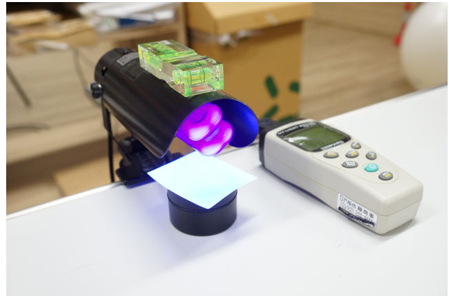
Figure 1: Experiment set up to measure the effect of UV mask.
