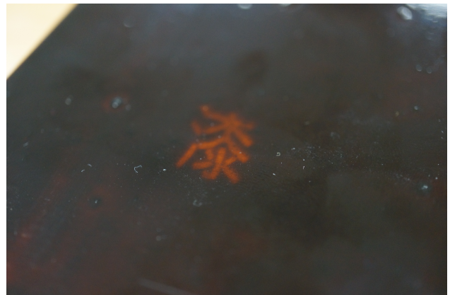
Figure 5: Result of UV laser system with Urushi on copper board.
