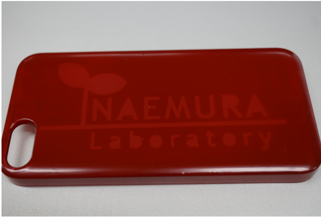
Figure 3: Result of UV lamp and paper method with red colored Urushi for iPhone case.
