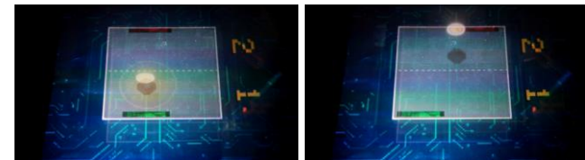
Figure 10: Motion of mid-air image. In left image, ball is in front and low position. In right image, ball is in back and high position.
