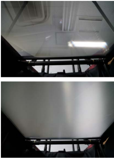
Figure 5 (Top) no louver film, (Bottom) with louver film
