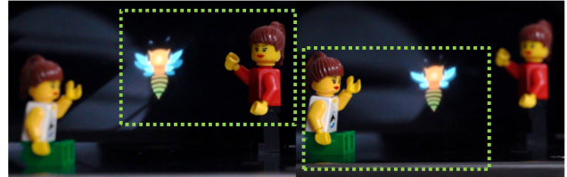
Figure 1: (left) Mid-air image formed at a 155-mm distance from MMAPs (A green rectangle shows a focus area is backward.) (right) Mid-air image formed at a 220-mm distance from MMAPs(A green rectangle shows a focus area is forward.)
