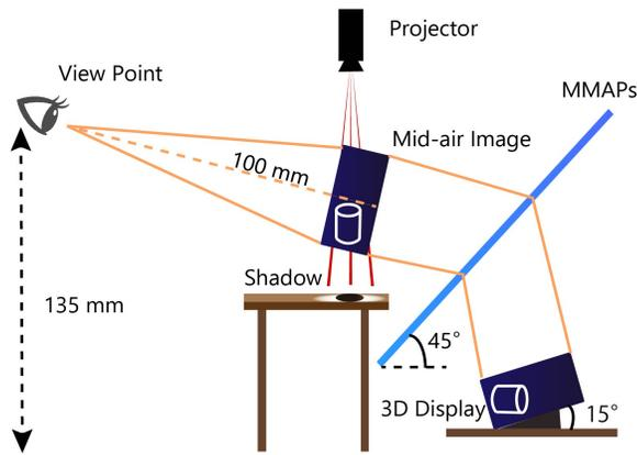
**Figure 2: System Design.** When the light incident on the MMAPs from the light source is reflected, the mid-air image is formed as a real image at the plane symmetry position. A shadow is projected directly below the formed mid-air image.
