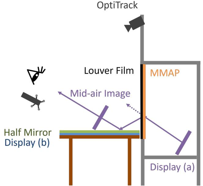
Fig. 3. Optical Design. Light from the display passes through the micro-mirror array plates (MMA) and is reflected by the half-mirror to form mid-air images. OptiTrack tracks the dynamic light source movement to provide real-time shading information.
