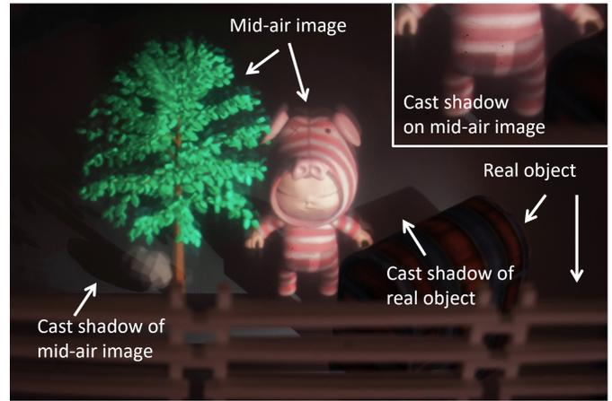
Fig. 10. An application in which the real object and the mid-air image seamlessly integrate through shadow representation. The shadow of the real object is projected onto the mid-air image.
