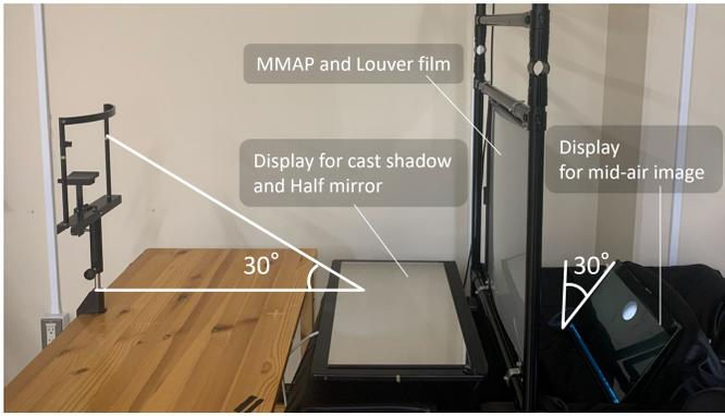
Fig. 6. Setup of the experimental apparatus. Participants fix their viewpoint on a head-chin rest and observe the mid-air image, which is tilted at a 30-degree angle.
