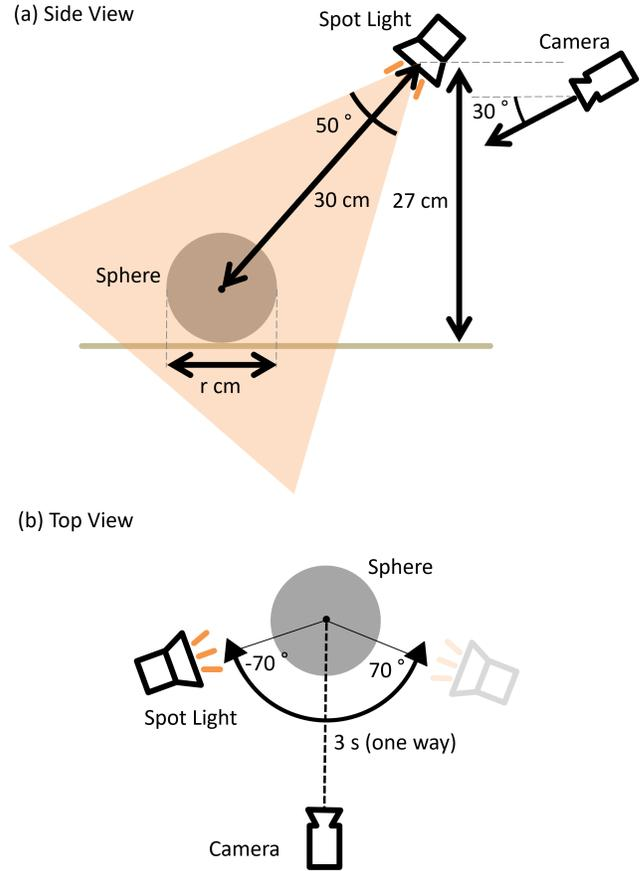
Fig. 4. Dynamic lighting configuration. The spotlight illuminates the CG object from a fixed height, always facing it, and moves along a circular arc.
